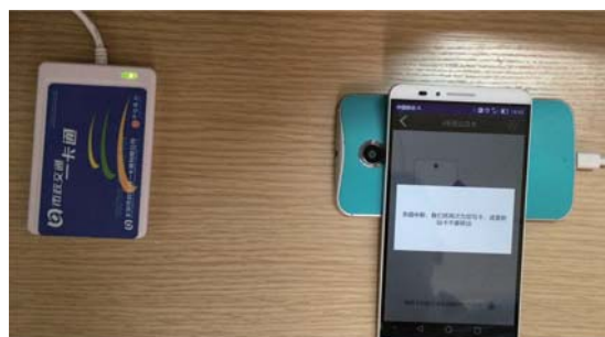
Fig. 3: Relay attack leads a fail top-up.
